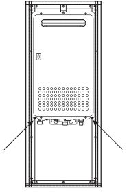
Figure 4: Location of lower mounting brackets.
