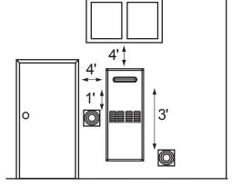
Figure 1: Discharge Vent Clearances.
